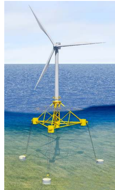
SBM Tension Leg Platform
